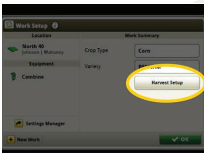
3) From here, select Harvest Setup to continue making adjustments to machine settings for crops and field conditions
