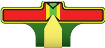
**Critical:** Draper belt tension indicator must be in the position shown to ensure proper draper function in all conditions
