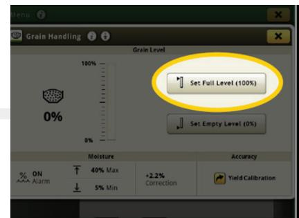
4) Once the grain tank is filled push "Set Full Level." Grain tank fill level is now complete
