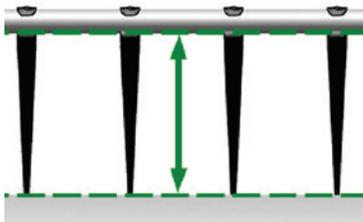
Reel finger pitch is adjustable. Adjustment levers are at both ends of the reel. A more advanced finger pitch helps pick up downed crop. A less advanced pitch reduces the material wrapping on the reel.
