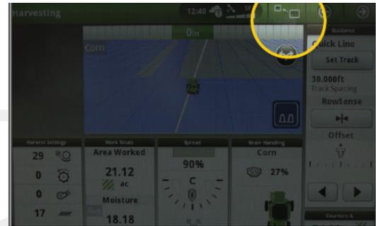
2) Hit the button to move that screen to the extended monitor
