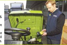
The CLARK handset can be used for diagnostics and settings of up to 20 different performance parameters to match your requirements.
