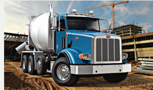
An advanced composite hood provides exceptional durability, and the stainless steel grille protects the cooling system. The dramatic slope of the hood improves forward visibility.
