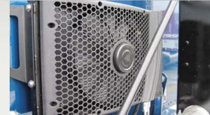
For optimal performance, the remote condenser and brushless fan assembly is centrally installed on the lower exterior wall of the sleeper.
