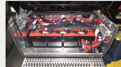
The battery box can be mounted in several locations in order to meet customer operational requirements.
