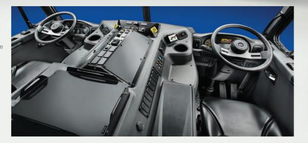
The 520 interior features an ergonomic dash design with LED backlit gauges, a driver information display for critical vehicle data and rocker switches within easy reach for maximum driver comfort and productivity.
