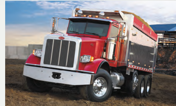
The 367's gently sloped, long-length hood not only enhances visibility, it allows for a 1,438-square-inch radiator to accommodate engines of up to 600 hp.
