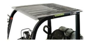
Cervus offers both overhead and full enclosure rain guards for your lift trucks. Rain guards are a practical and economical way to protect forklift operators from rain or sun. Keep your lift trucks moving and your operators comfortable and productive.
